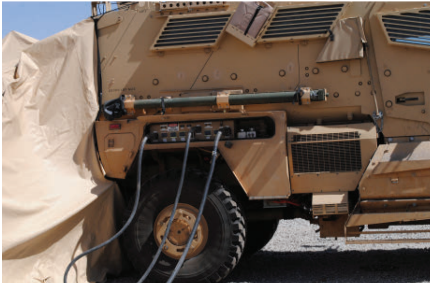
The OBVP power-generation system creates power at the vehicle transmission, and can provide 55 to 120 kilowatts of power — far more than a typical vehicle alternator.
